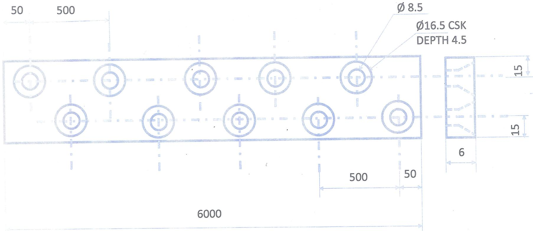
NOTE : PITCH IN BETWEEN TWO HOLES IS 500 THROUGH OUT LENGTH.AS PER SHOWN IN DRAWING
